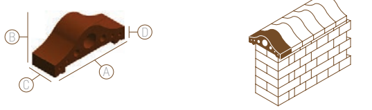
Harpuşta Oval Pres Tuğla // Saddleback Coping Elliptical Facing Brick
